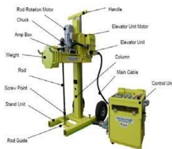
Fig. 1. A typical Screw Driving Sounding (SDS) equipment.
