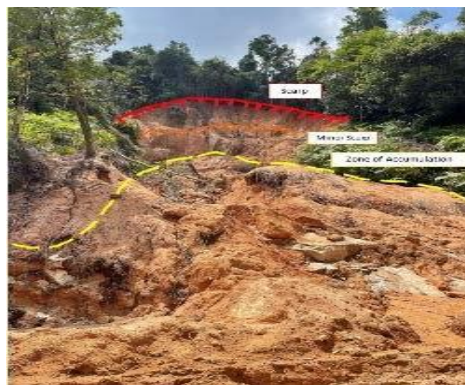
Fig. 1. Rotational landslide with huge soil and small boulder accumulation at the toe slope.
